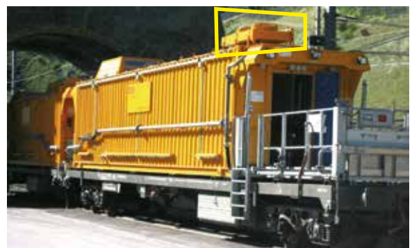
Radiator mounted separately on wagon roof
